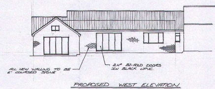
PROPOSED WEST ELEVATION
