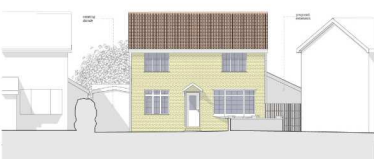
ELEVATIONS : North East scale : 1 : 100
